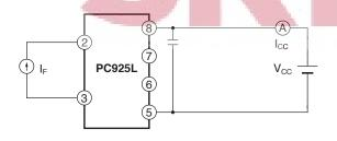
Fig.6 Test Circuit for UVLO Threshold
