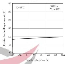
Fig.25 Relative UVLO Threshold vs.
